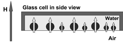
**Fig. 1.** Super-paramagnetic colloidal particles confined at a water/air interface due to gravity. The curvature of the interface is actively controlled to be completely flat; therefore the system is considered to be ideal two-dimensional. A magnetic field  $\mathbf{H}$  perpendicular to the interface induces a magnetic moment  $\mathbf{m}$  in each bead leading to a repulsive dipolar interaction.
