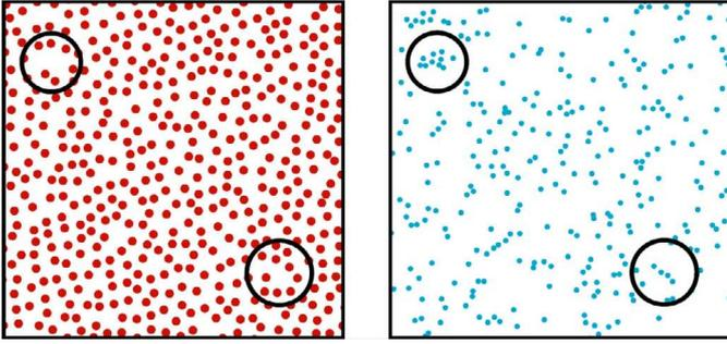
**Fig. 2.** Snapshot of a particle configuration ( $\Gamma = 5$ , relative concentration  $\xi = 41\%$ ) where big (left) and small (right) particles are displayed separately. The clusters of small particles (right) fit in the voids formed by the big particles (left) as highlighted by circles for two examples.
